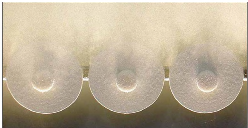
Fig. 5 Ceramic membrane discs working as gas diffusers
