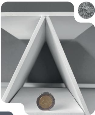
Fine grainsized porous high alumina ceramic plate with a brought field of applications and outstanding properties
